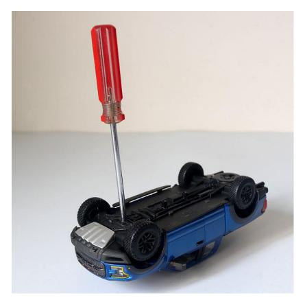
Use a phillips-head screwdriver to remove the body from the chassis.
