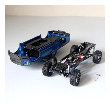
Install the electronics, (Electronics (Servo, Battery, Speed Control and Receiver) sold separately)
