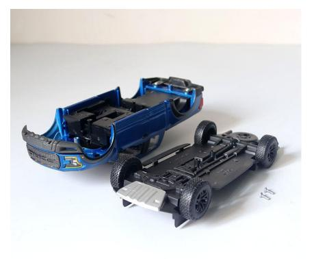
Use a hobby knife remove excess material from underneath the bed of the truck.
